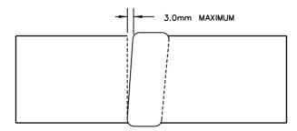
MOULD SQUARENESS AND ALIGNMENT ARE MEASURED AT THE WELD COLLAR ON THE UNDERSIDE OF THE RAIL.
