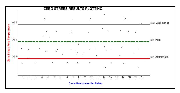
Figure 19.3: Zero Stress Results Plotting
