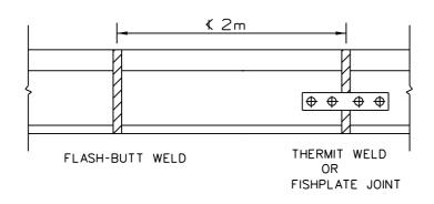
MINIMUM DISTANCE BETWEEN THERMIT WELD/JOINT PLATE JOINT AND FLASH-BUTT WELD MUST BE AT LEAST 2m. ANY DEVIATION MUST BE APPROVED BY THE DEPOT ENGINEER PERSONALLY.
