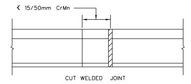
IF WELD IS DEFECTIVE, CUT RAIL NOT CLOSER THAN 15/50mm CrMn FROM THE CENTRE OF AN EXISTING WELDED JOINT. IF WELD IS SOUND, THE CUT MAY BE MADE THROUGH THE WELD.
