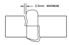
MISALIGNMENT IS MEASURED AT THE WELD COLLAR ON THE UNDERSIDE OF THE RAIL.
