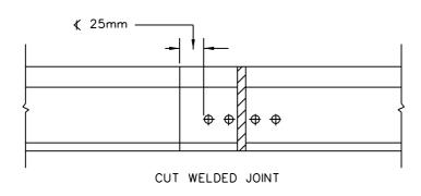
CUT RAIL NOT CLOSER THAN 25mm FROM THE EDGE OF AN EXISTING JOINT PLATE HOLE.
