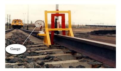
Fig 19.1: The Lifting Frame
