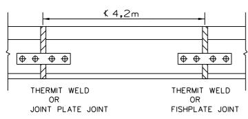
MINIMUM DISTANCE BETWEEN THERMIT WELD/FISHPLATE JOINT AND THERMIT WELD/JOINT PLATE JOINT MUST BE AT LEAST 4,2m.
